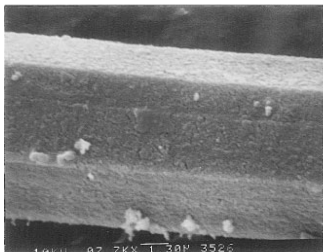
Figure 5. Scanning electron micrograph of a ceramic particle obtained by heating a single crystal of 1 to 1200 °C under argon for 1 h.
